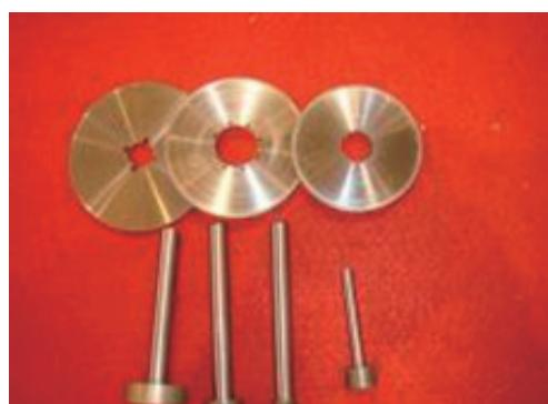
Electroplated diamond/CBN wheels for grinding, groove finishing, diamond polishing and other wheels with complicated profile for the application of metal and nonmetal.
